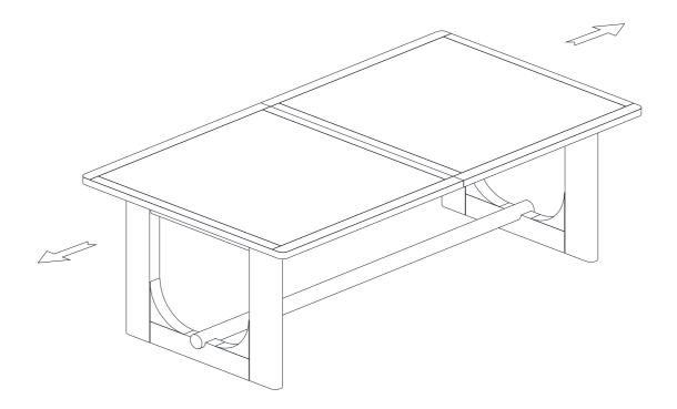
• Then fold out the leaf as shown below. Push the table top close firmly, then lock all 4 latches, before use.
